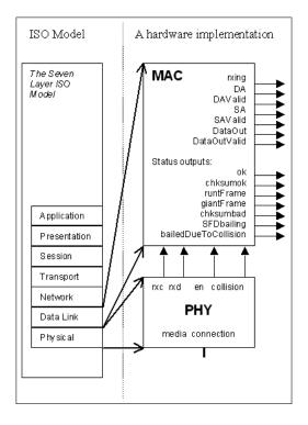
The diagram shows the ISO seven layer reference model on the left. On the right is a block diagram of the hardware for the two layers which are of concern for this design. Note that the specific inputs and outputs are not part of the ISO specification. For this design project we are assuming a PHY device of a particular kind and we are assuming that certain types of outputs are required from the MAC ... your design needs may differ.
