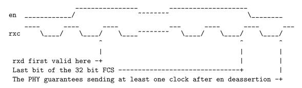
In summary, at a minimum this MAC layer must continuously monitor the four signals from the PHY and extract data and perform the following checks that should be performed:
